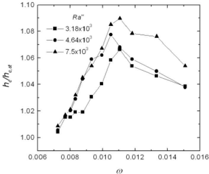
Figure 9- Heat Transfer Enhancement for Different Heat Inputs [2]
