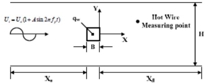
Figure 1- Concept of Oscillating Flow Experiment [1]
