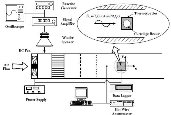
Figure 2- Schematic of the Oscillating Flow Experiment [1]
