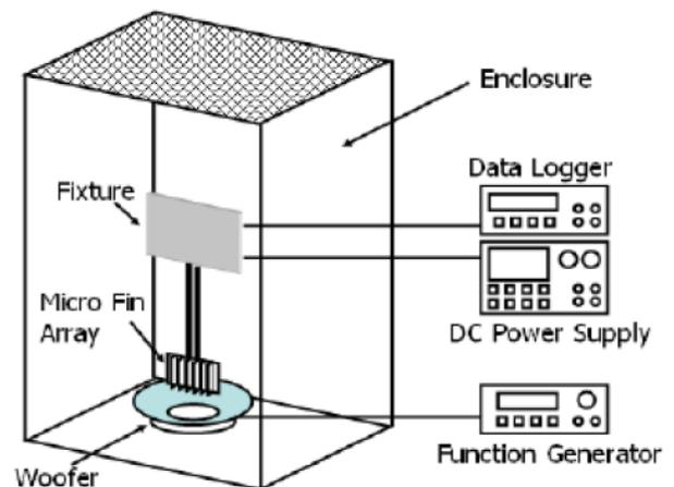
Figure 6- Natural Convection Experiment with Loud Speaker Excitation [2]
