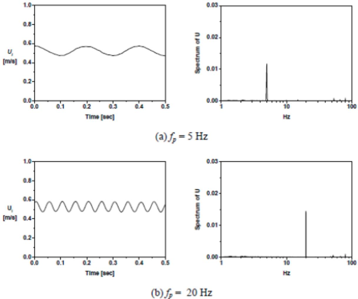
Figure 3- Periodic Motion of Flow and Its Spectrum [1]
